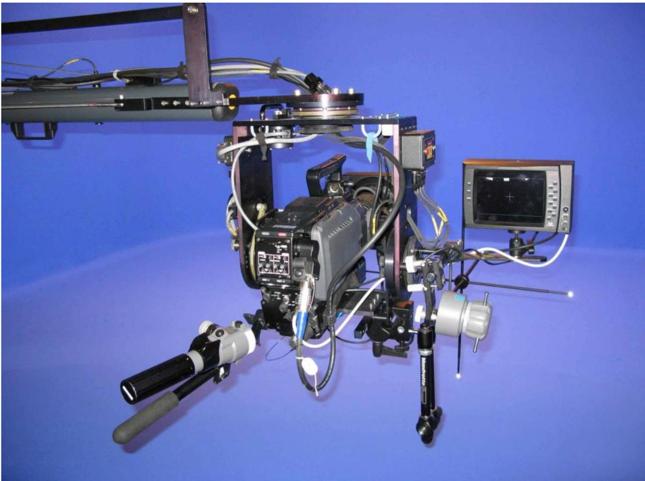
The “PRIMA MV” manual operating head is mounted on the crane upside down. In this manner the arm is never an obstacle to the head movement that can easily make 360° and more. The cameraman can start from the floor with a very low point of view.
