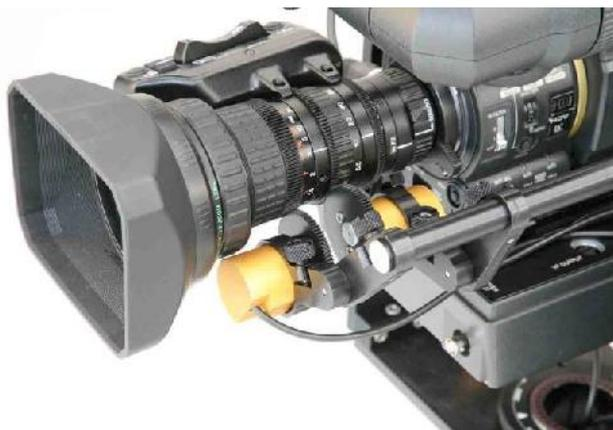
For the lenses that has not the encoders inside there are external encoders to read the zoom and focus position.
