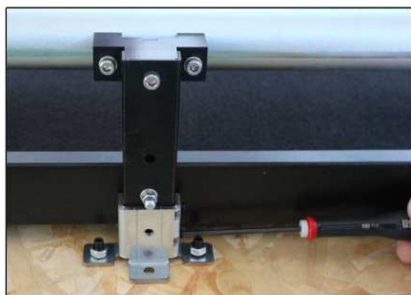
Fix the screws to the crossbar
