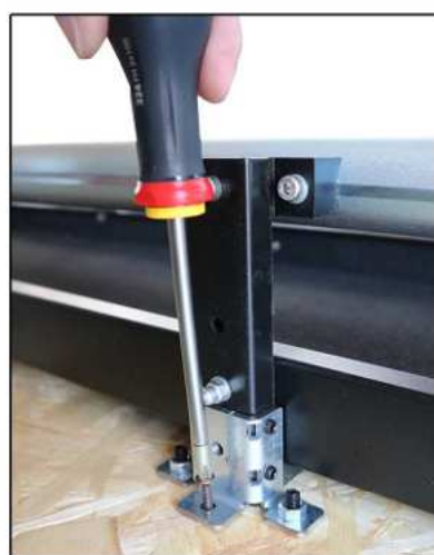
Screw the wood screw. The hole is diameter 6
